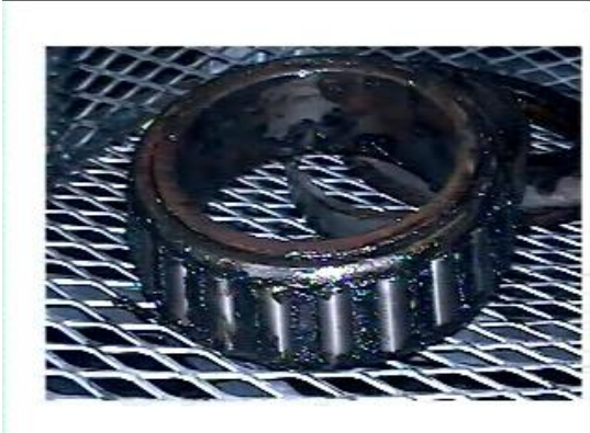
Bearing Before Cleaned With Pure Clean
